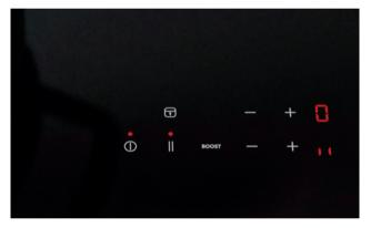
When you press the **pause** function, all activated zones are paused – and when you press the pause button again, the zones will come back to the same temperature as before. That way you can suspend the cooking process if you're interrupted, and re-start again in an instant.
