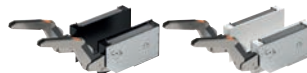
UTRUSTA hinge with damper for horizontal door, 2-p. This hinge has an integrated damper, so that the door closes slowly, softly and silently. You can easily mount the door front in the right position, because the hinges are adjustable in height, depth and width. Snap-on hinges can be mounted onto the door without screws, and you can easily remove the door for cleaning.
