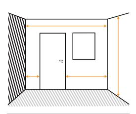
**01** Start by measuring from the floor to the ceiling. Then the distance between walls and from the corners to the doors.
