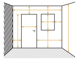
**02** Measure each window including the frame and their distances from the floor, the ceiling and the corners of your room. Do the same for the door(s).
